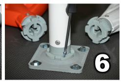
With a philips screwdriver, install the 5/8" set screw to lock in securely
