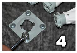
Place the base plate over holes and use a socket wrench with a 1/2" drive to thread all four lag screws
