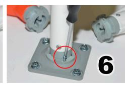
With a philips screwdriver, install the 5/8" set screw to lock in securely
