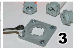
• Place the base plate over the four holes and use a socket wrench with a 9/16" drive to thread all four wedge bolts
