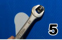
• Use a 1/2" wrench or socket to tighten flange nuts to hold sign in place
